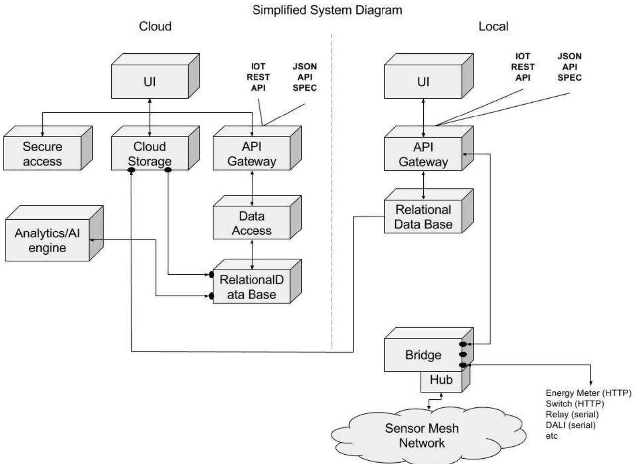
Fig. 5 Simplified System Diagram. HVAC and BMS systems access to data through REST and JSON APIs in both cloud and in-building systems. This provides both data access, access to predictive analysis and fine grained (area/room/device level) control if desired.
