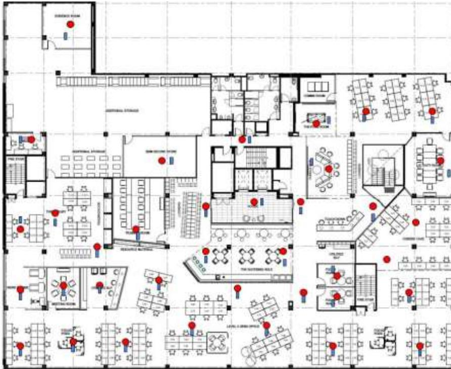
*Fig. 3 Example Sensor layout. The sensors are distributed to give excellent coverage and notification in doorways, hallways and work areas. Sensor numbers (density) can be increased or decreased to add finer resolution, however there is diminishing benefit as sensor ranges overlap and for most cases the ranges do not have to be contiguous.*
