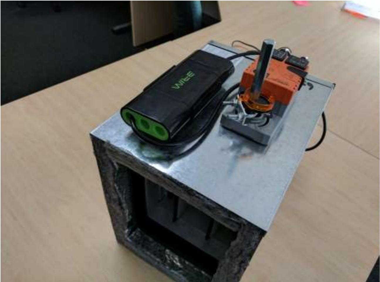
*Fig. 6 A sensor-controller configured at the lowest level to add semi-autonomous VAV control at the room level. The VAV can then react to local physical events including temperature, emergency, occupancy etc as well as be driven to participate in near real-time load shedding and shifting.*
