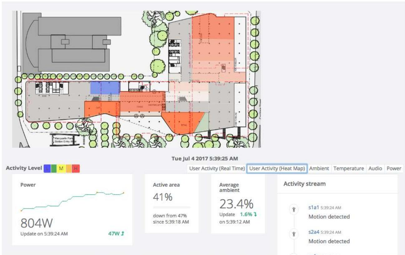
Fig. 4 Usage heat maps per area. This feedback can be supplied to the HVAC control system to fine tune and minimise where air conditioning is used. This can be further refined
